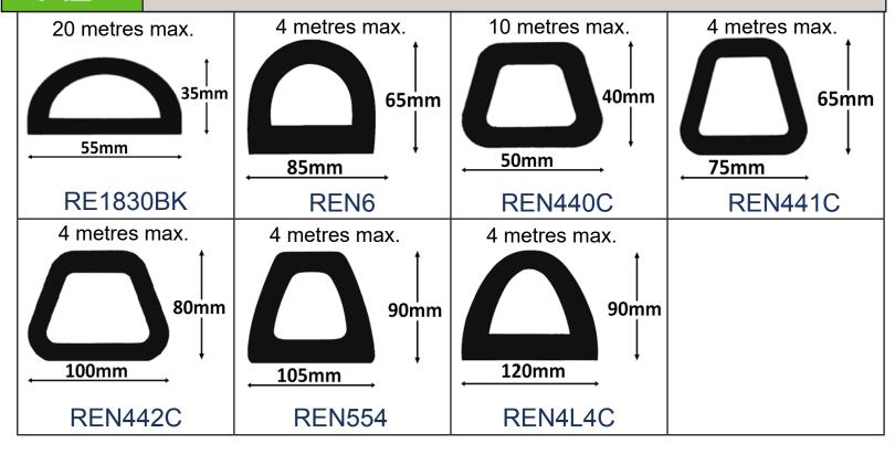
Fender rubber is used to lesson shock or damage to wharfs, boats/ships. It's also used within the transport Industry as a buffer on the backs of truck or loading bays.
