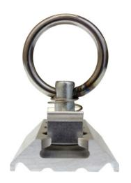
The **Ally-cargo track anchor system** withstands up to 1000kg vertical force on track and ring restraint when used together. It withstands up to 350kg force (at 45 degree angle) on track and ring restraint when used together.
