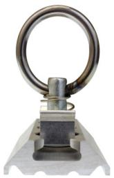
The **Ally-cargo track anchor system** withstands up to 1000kg vertical force on track and ring restraint when used together. It withstands up to 350kg force (at 45 degree angle) on track and ring restraint when used together.
