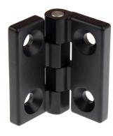
AS-AZ2510B 50mm X 50MM open 4mm thick Die cast alloy 4 hole x 6.3mm dia. Counter sunk Fixed pin Stainless steel 304
