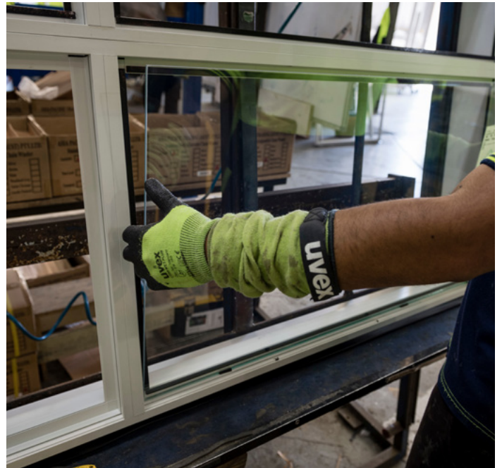
tesa® 60402 seals and cushions the glass onto the frame
