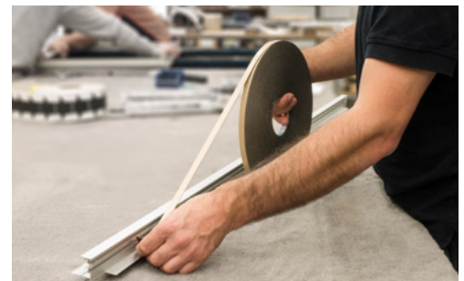
tesa® 60402 applied to aluminium frame
